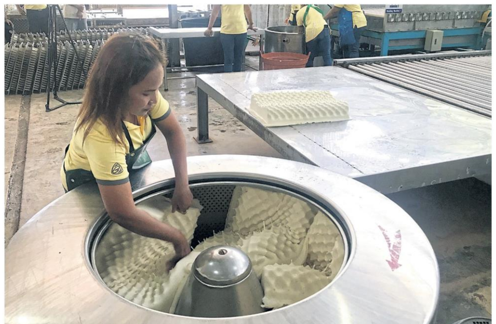
RIGHT Pillows are spun in the machine until almost dry.
