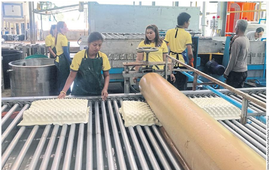
ABOVE Each pillow is pressed to remove water after being washed.
