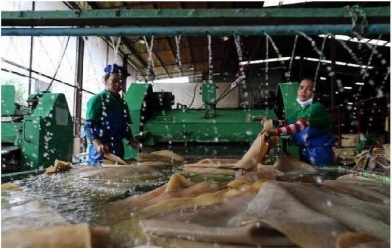
shaping up: Workers handle rubber sheets as they pass through a rubber sheet washing machine at the Thai Hua Rubber factory in Rayong province. Photo: Bloomberg
