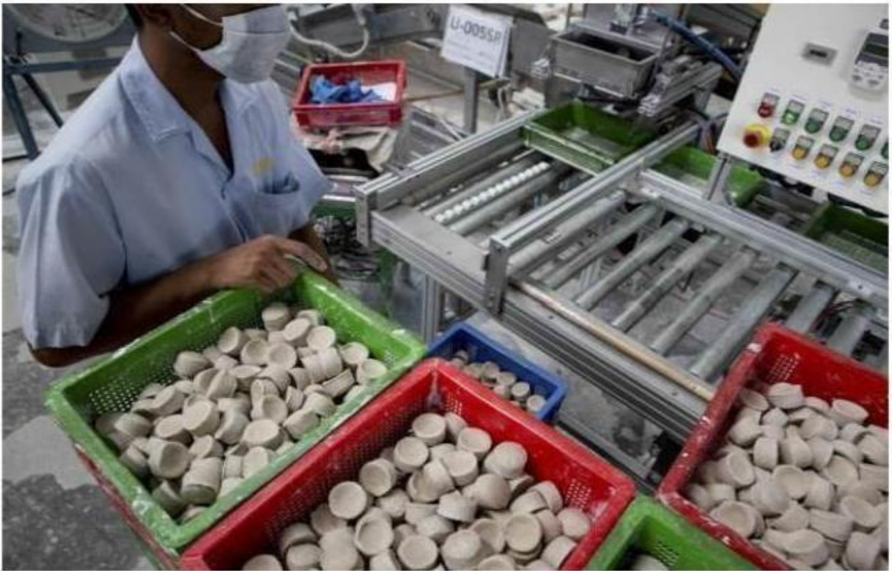
a new ball game: Raw rubber before it is shaped and turned into a pressurised core called a slug at a Wilson tennis ball factory outside Bangkok. Photos: © 2017 The New York Times
